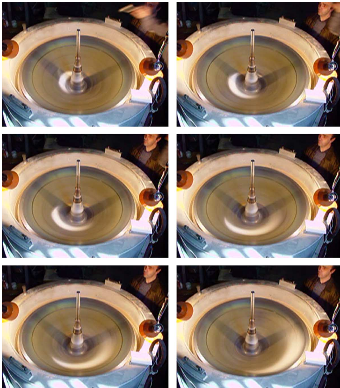
Fig. 2. An illustration of the gibbsite powder movement over the rotating conic plate (the sequence of the pictures with the time delays 0.12 s).
